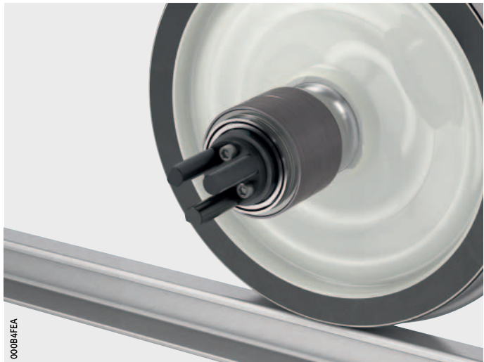
Figure 49 Unscrewing the guide bush from the shaft journal
