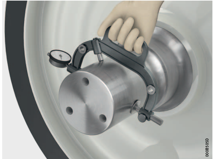
Figure 31 Measuring the shaft journal using the snap gauge
