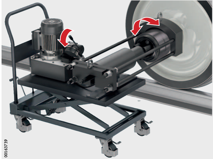
Figure 38 Extractor shoe in contact with shaft
