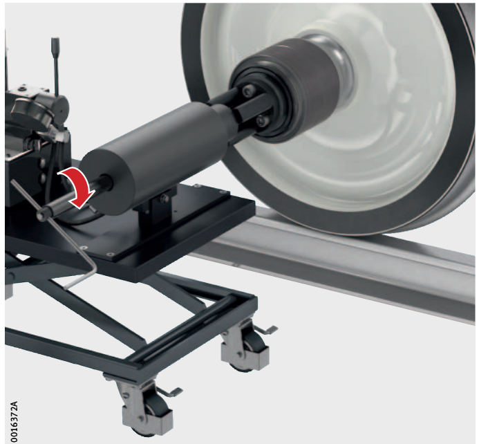
Figure 37 Screwing the spindle into the guide bush
