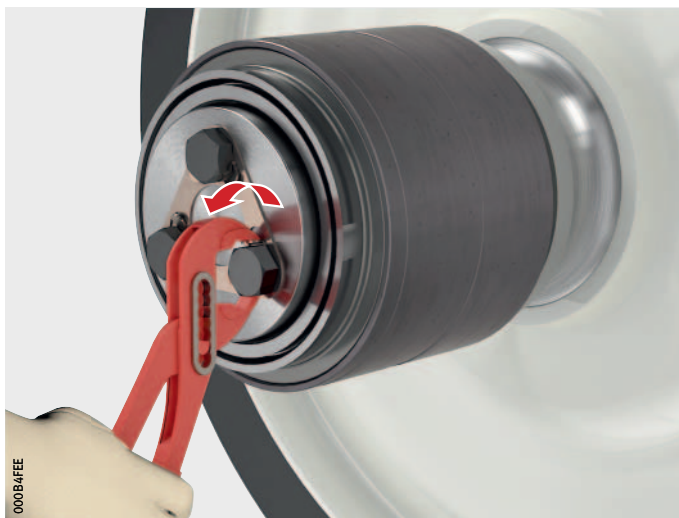
Figure 51 Bending back the tabs on the tab washer
