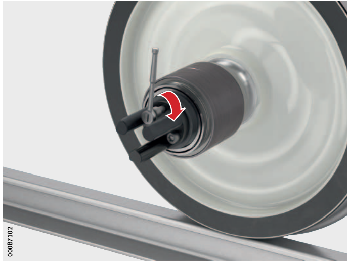
Figure 34 Screwing on the guide bush
