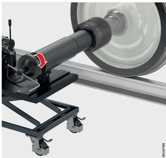
Figure 46 Screwing the spindle into the guide bush
