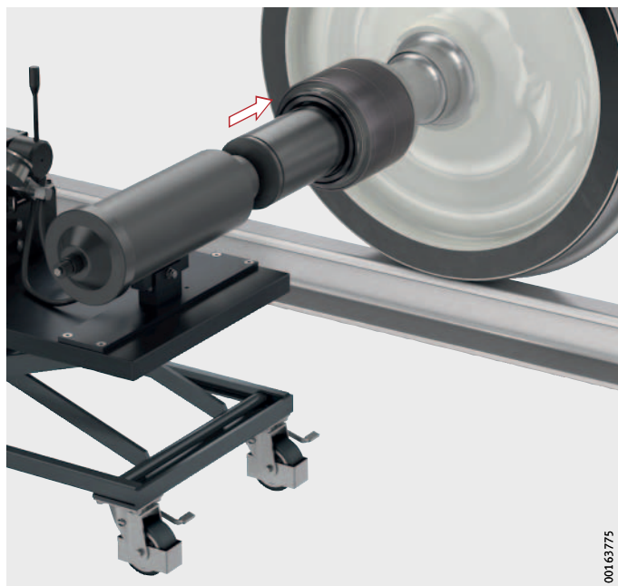
Figure 45 Aligning the hydraulic unit to the TAROL unit
