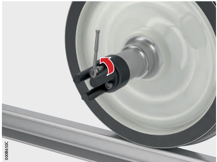
Figure 39 Unscrewing the guide bush
