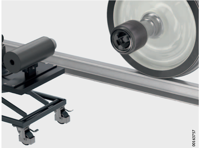
Figure 43 Moving the hydraulic unit into place
